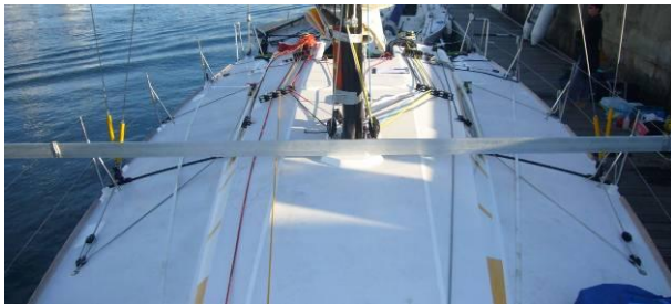
Photos 9 and 10: Examples of the placement of the bar for measuring mast base height
