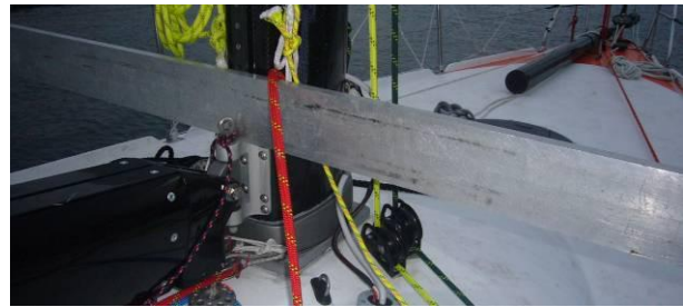
Photos 9 and 10: Examples of the placement of the bar for measuring mast base height
