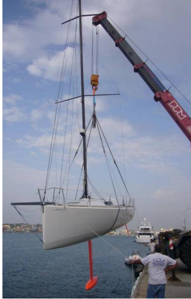
Photo 1: Lifting with strops
