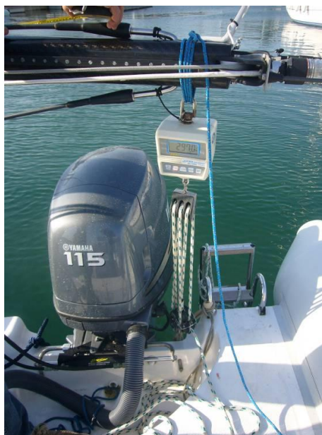
Photo 8: Load cell in place
