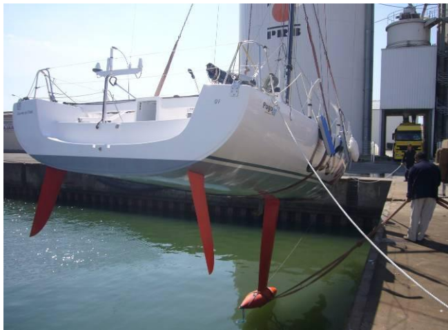
Photo 6: Lowering of the boat with tension on bulb
