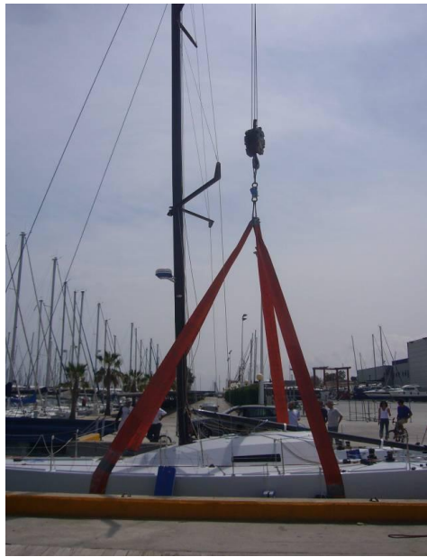
Photo 2: Lifting with long slings
