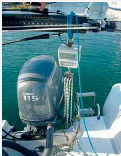
load cell in place
