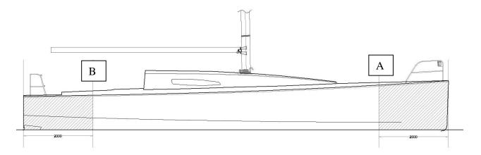
The topsides are defined as the hull surface between the **waterline** and the **sheer**.
