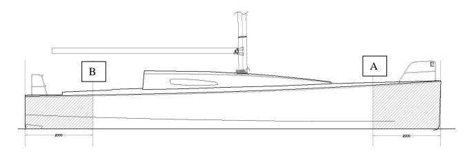
The topsides are defined as the hull surface between the waterline and the sheer.
