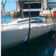
Boat in the water with bulb sling held tight
