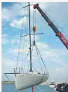
Lifting with strops
