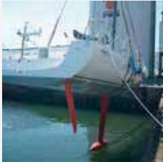
Lowering of the boat with tension on bulb
