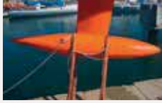
Bulb protruding at the front with aft line to remove sling + line in the middle to hold slings in place
