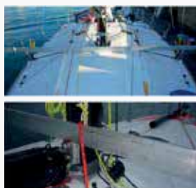
Examples of the placement of the bar for measuring mast base height
