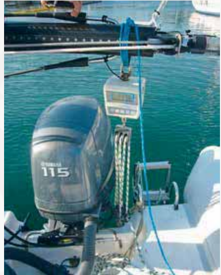
load cell in place
