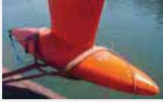
Bulb protruding at the front with aft line to protect the trailing edge, and forward line to remove sling
