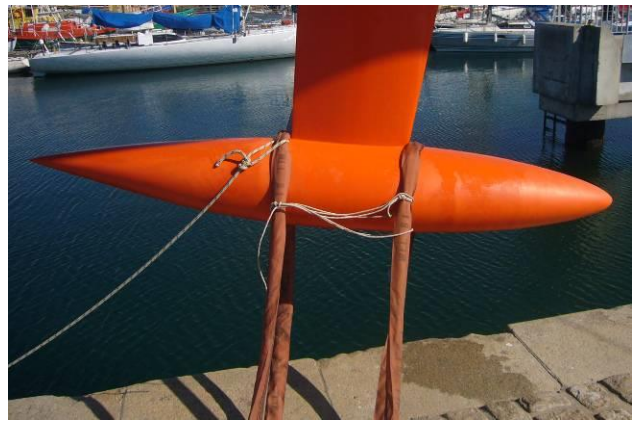
Photo 5: Bulb protruding at the front with aft line to remove sling + line in the middle to hold slings in place
