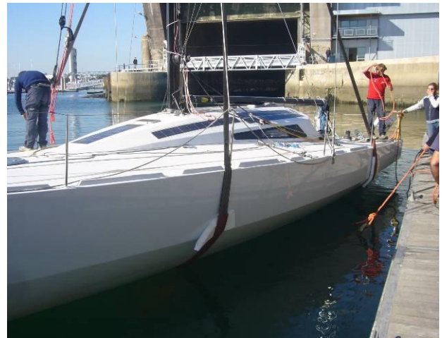
Photo 7: Boat in the water with bulb sling held tight
