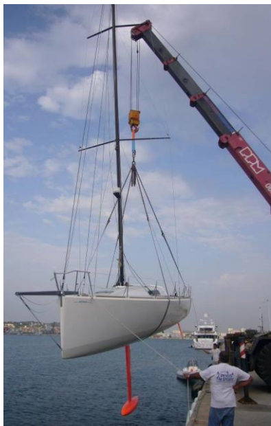
Photo 1: Lifting with strops
