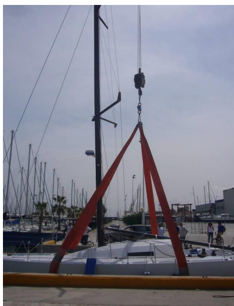
Photo 2: Lifting with long slings
