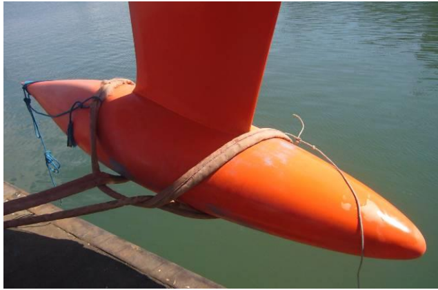
Photo 4: Bulb protruding at the front with aft line to protect the trailing edge, and forward line to remove sling
